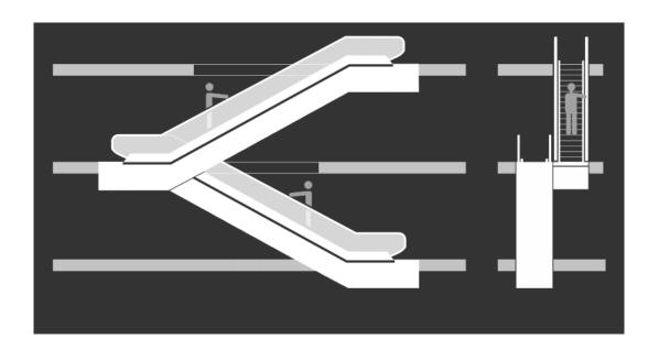
The escalator that connects subsequent levels in one-way traffic is used mainly in small department stores and commercial centers.
