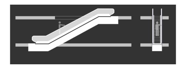
The escalator connects two levels. It is used in objects in which persons travel in one direction mainly. A flexible directional operation is possible (e.g. travel in one direction in the morning, and in other direction in the afternoon).
