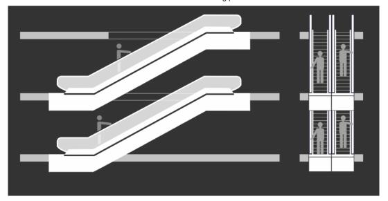
The escalator that connects subsequent levels in a non-continuous two-way traffic is used in department stores, office buildings and public transport objects. With multiplication of this operation arrangement there can be used sequence operation: travel in a defined direction depending on day time.
